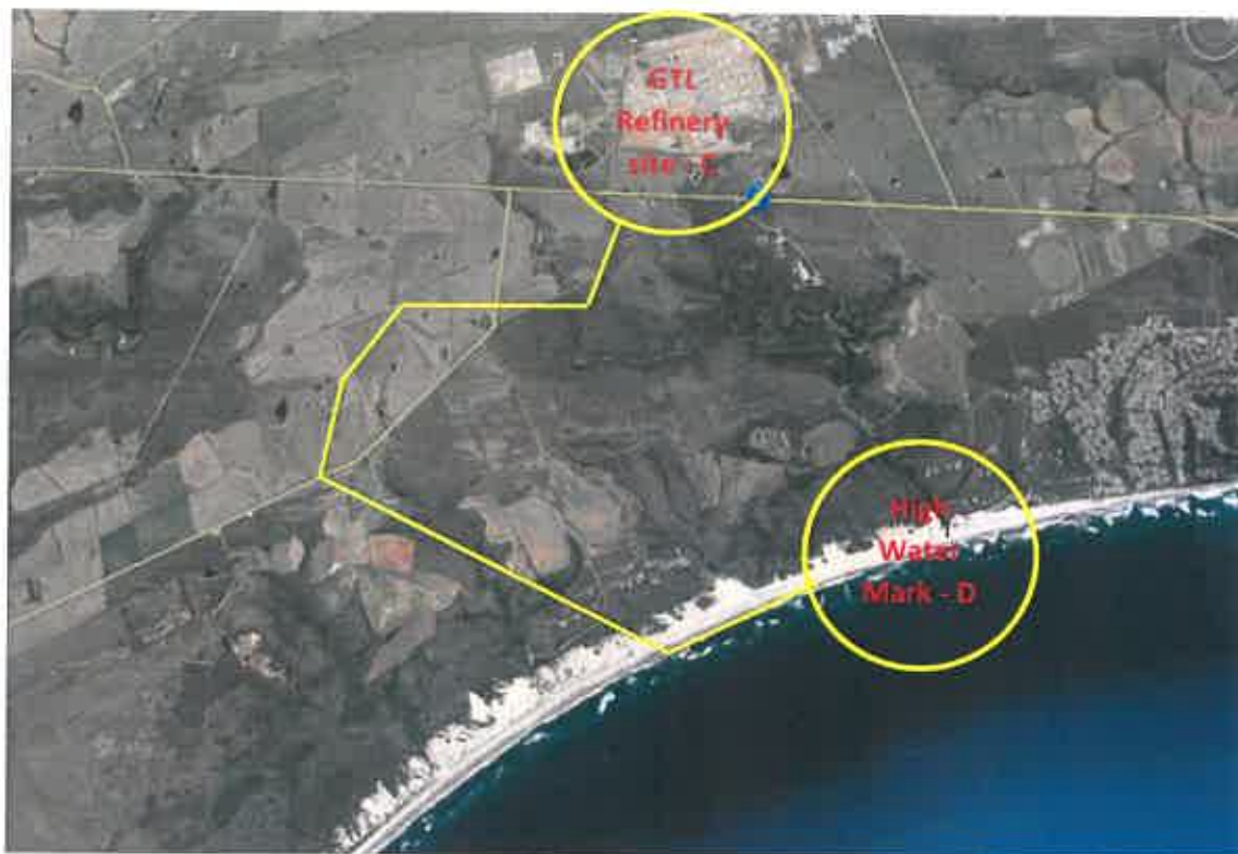
Figure 2: Layout of the pipeline (7.1km) from the refinery to the high water mark (Point C is the GTL Refinery plant and Point D shows the High water mark)
